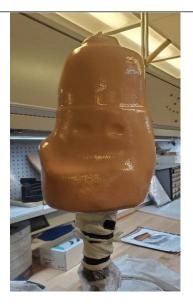
6. Once the lamination has cured, cut out and shape your trimlines. Beware to not sand too much of the punch holes as this might affect the locking in mechanism.
